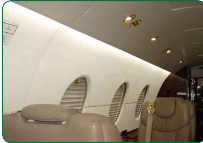
B400A interior with EMTEQ LED lighting
